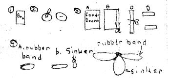
Put rubber band through hole in sinkor.
